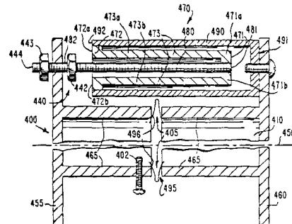
the bilateral ground planes coincident with each section. The dielectric separating each stripline from the ground plane is modified in the region in the perforations to reduce the dielectric constant in the region.
